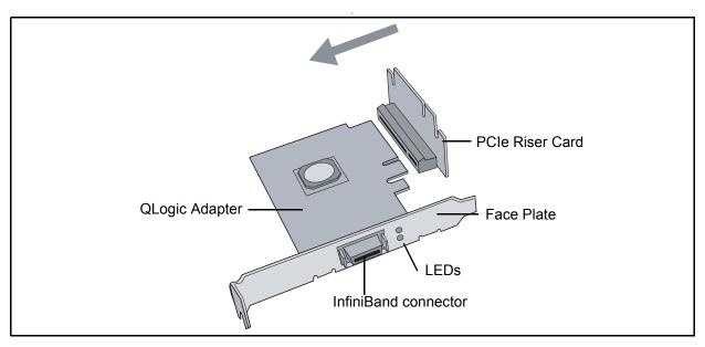
Figure 4-5. QLogic PCIe HCA Assembly with Riser Card
